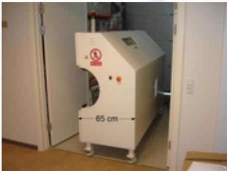
*Width of the X-ray cabinet when disassembled is only 65 cm - it passes easily through a standard office door*
